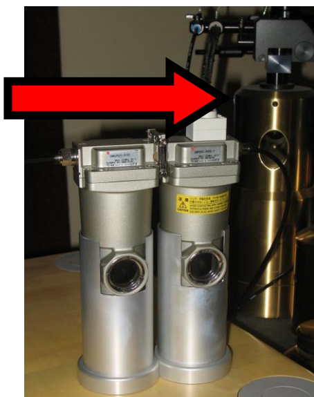
Fig. 7. Silver filters- see arrow for airflow
