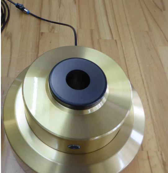
Fig. 10. Base with airbearing
