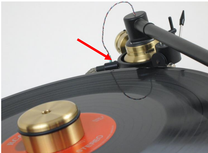
Fig. 4. See cable fixing.
