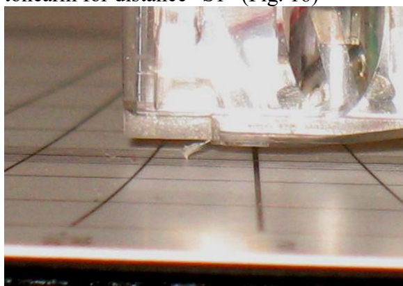
Fig.16. Stylus tip is in front of zero point B.
