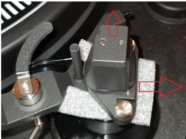
Fig. 6. Arm tower-removing transport foam
