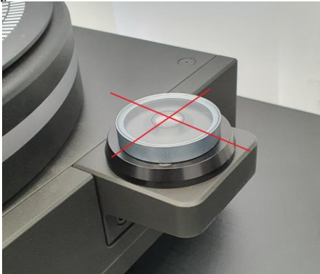
Fig. 15. Leveling on arm base only
