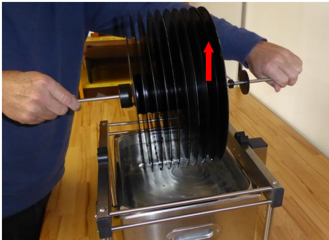
Fig. 10.0. Lifting spindle with LPs out of bath.
