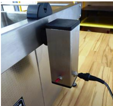
Fig. 5.0. Motor, switch, plug in DC supply
