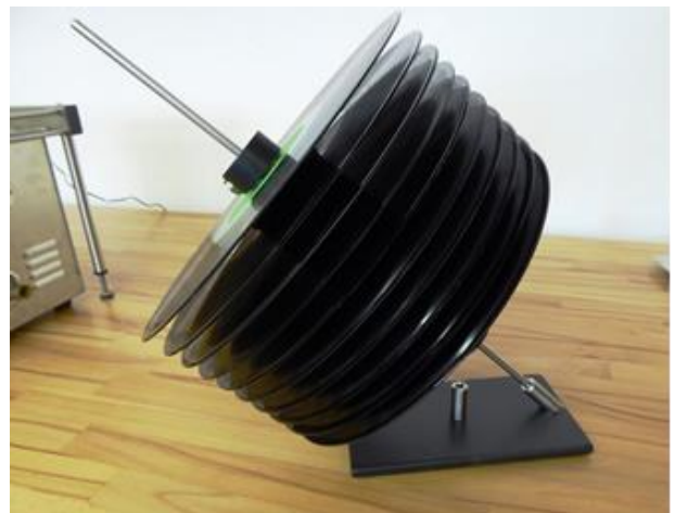
Fig. 10.2. Spindle with records drying in the stand
