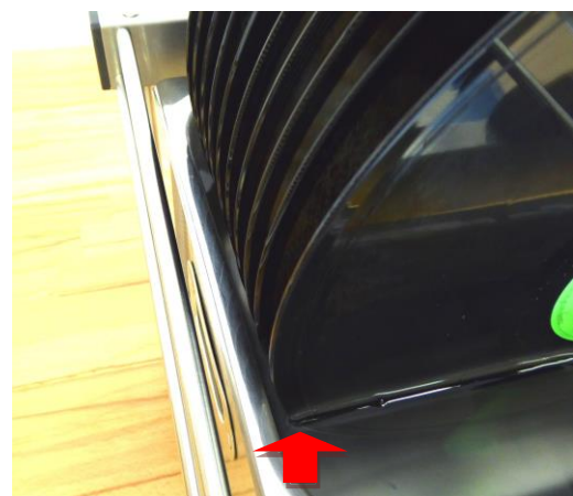
Fig. 9.5. Gap between edge of bath and LPs
