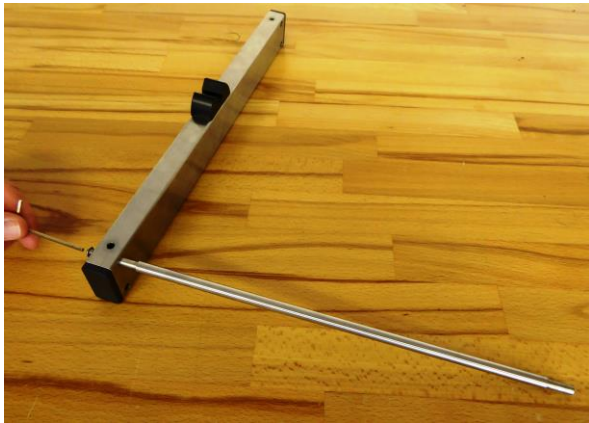
Fig. 2.2. Fixing rod into square tube
