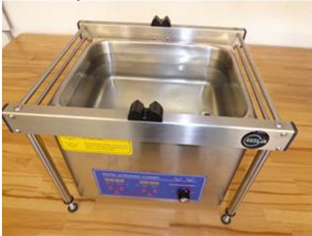
Frame is positioned over ultrasonic (US) cleaner bath
