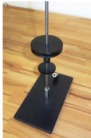
Fig. 6.1. Spindle with first spacer
