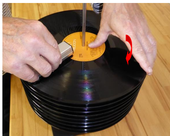
Fig. 11.1. Wiping LPs with carbon brush
