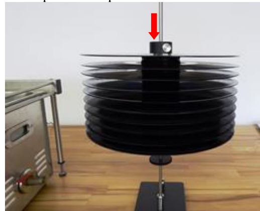
Fig. 7.3. Spindle fully loaded with 10LPs
