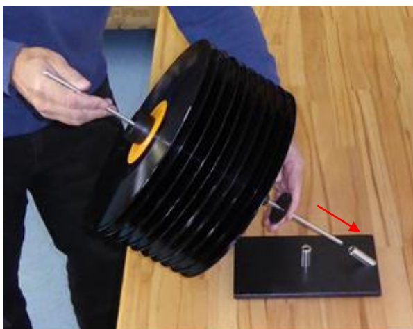
Fig. 10.1. Inserting spindle in the stand
