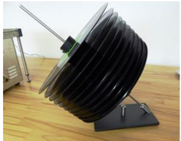
Spindle with records in drying position
