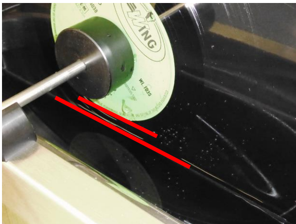
Fig. 9.4. Water level below record label.
