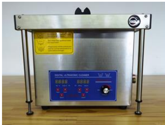
Fig.4.3. Level frame with US cleaner bath
