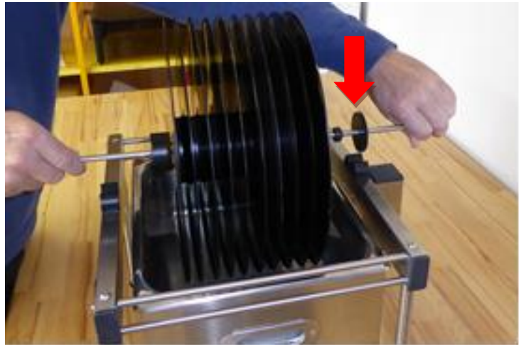
Fig. 9.1. Lowering spindle in the rotation position
