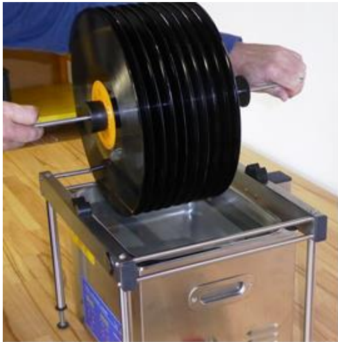
Fig. 9.0. Holding spindle with LPs
