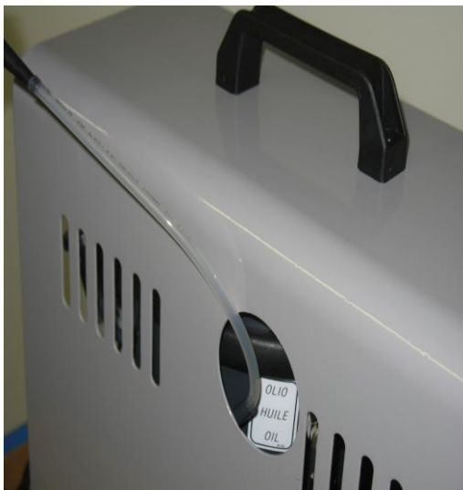
Fig.4 Oil filling from side of the compressor
