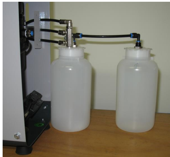
Fig.5. Double drain PVC bottle system
