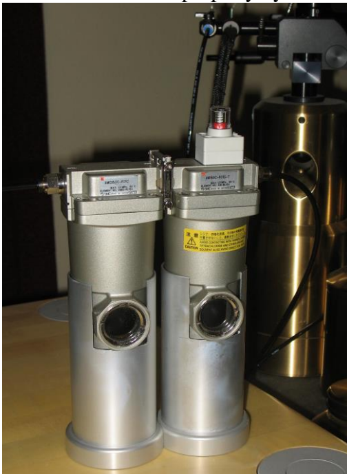
Fig.6 Silver filters-dryers- see arrow for airflow
