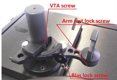
Fig. 5. Arm tower- various adjustments
