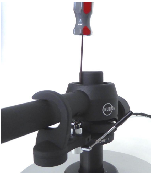
Fig. 12. Adjusting VTA screw
