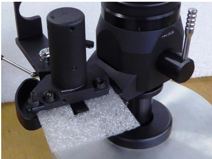
Fig.14. Insert fixing foam by lifting horizontal tower- see Fig. 2A
