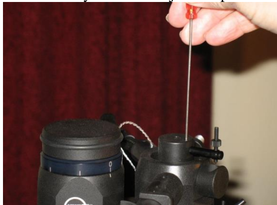
Fig.10 Fixing vertical damping holder
