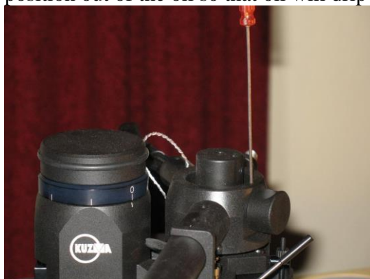
Fig.11 Removing vertical trough
