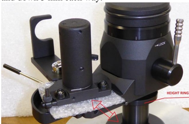
Fig.2A. Pull out fixing foam on the horizontal bearing assembly
