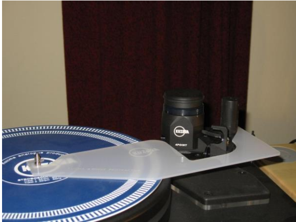
Fig.3 Protractor for pivot to spindle distance
