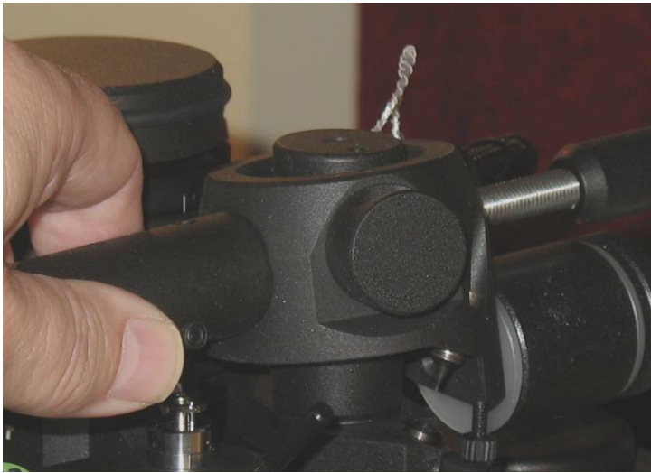
Fig.4. Assembling the tube onto the horizontal bearing tower.
