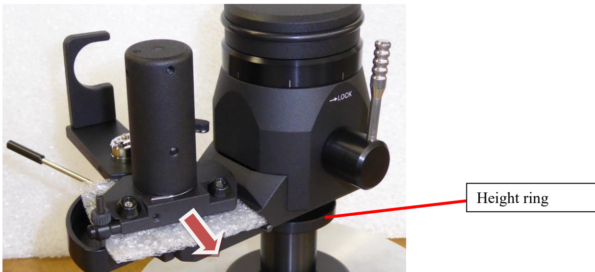
Fig.3. Pull out fixing foam on the horizontal bearing assembly
