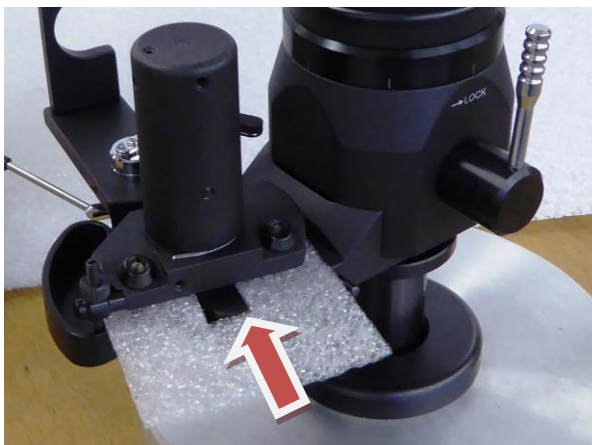
Fig.16. Insert fixing foam by lifting horizontal tower- see same Fig. 3
